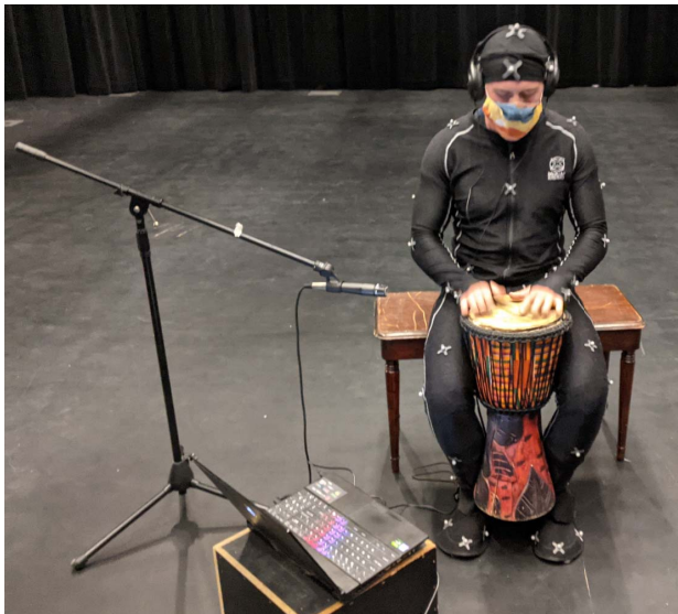
Figure 4: The Motion + Audio Capture setup. A Qualisys motion capture system was used to record player motion, and the drum audio was recorded into Ableton Live.
